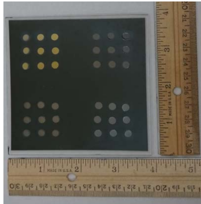
Figure 2.20. Metal contacts (monolithic 3 \times 3 arrays) on 10 \times 10 \text{ cm}^2 ( 4 \times 4 sq. inches) ^{10}\text{B} -doped Se (As, Cl) detector fabricated on \text{Al}/\text{Al}_2\text{O}_3 substrate. Upper left: gold (Au); upper right: nickel (Ni); lower left: tungsten (W); and lower right: palladium (Pd).
