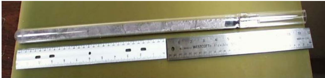
Figure 3.2. Zone refined (ZR) Cd ingot within a quartz ampoule; pure precursor material is on the right side while segregated impurities are on the left side of the ampoule.
