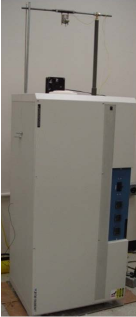
Figure 3.10. Picture of in-house growth furnace (left) with custom electronics for controlled pulling and rotation of the growth ampoule to ensure crystal quality and homogeneity. Custom pulling and rotation was installed, along with automation via H-Bridge motor controller and Arduino microcontroller.
