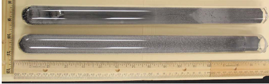
Figure 2.3. ZR a-Se ingots ( \sim 7N ) in quartz ampoules after multi-pass zone purification.
